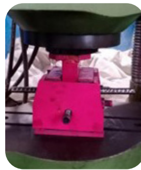
Shear testing of rebar
